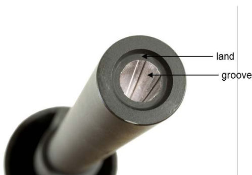
Figure 4: Rifling with grooves and lands labeled.
