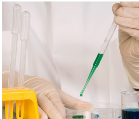
Figure 3: Disposable pipettes aid in accurate measuring of small volumes of liquids. It is important to use a new pipet for each chemical to avoid contamination.
